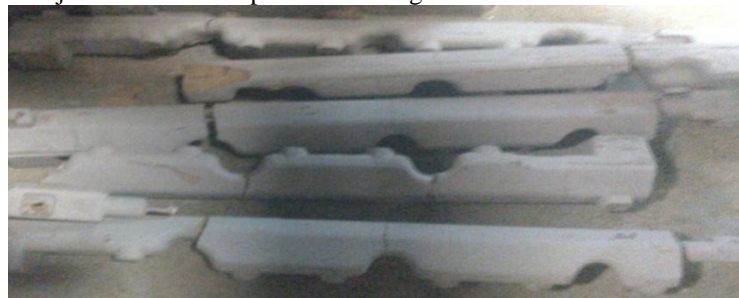
Figure 3 Cracked and twisted water jacket core
