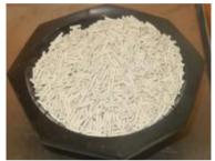
Fig 3. ZSM-5 Zeolite pellets
