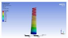
Fig.11 Maximum shear Stress
