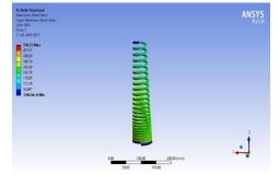
Fig. 3 Maximum shear Stress
