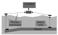
Figure 7: WSN checking framework for checking underground pipeline leak.
