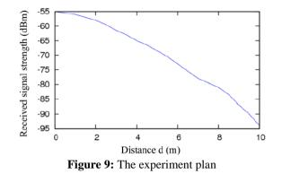
The experiment plan is shown in figure 9. The distance between the two sensors was increased until they could not communicate.
