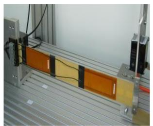
Figure1: Flexible Macro Fiber Composite (MFC) sensors
