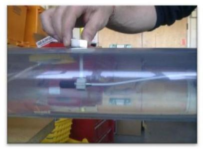
Figure 2: Pipe leak detection and localization method based on acoustic emission
