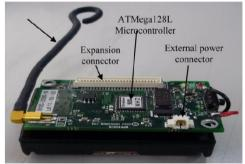
Figure 5: AMICA2 board has an extension connector which associates with sensors
