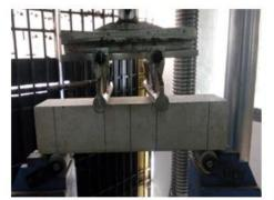
Fig.5 Flexural Strength testing
