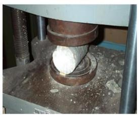
Fig.3 Split Tensile testing
