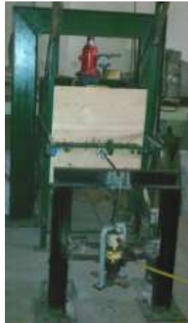
Figure (3): An overall view of the pull-out testing device used in the current study.
