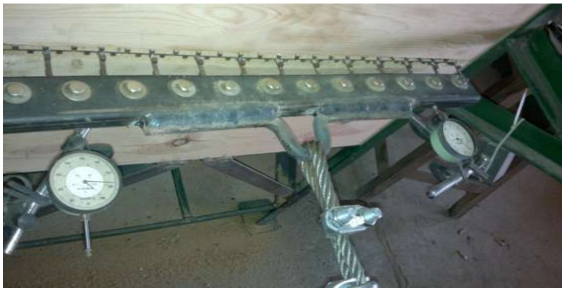
Figure (2): A photo shows the steel channel clamp utilized for holding the geogrids.
