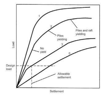
Figure 2 Load-settlement curves (Poulos, 2001)
