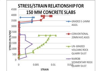
Fig.1.stress /strain relationship forcrushing of 150mm concrete slabs.
