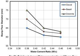
Fig.(3): Relation between Water cement ratio and Slump flow Diameter for Different Types Aggregates
