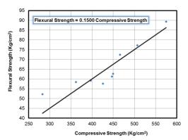
Fig.(11): Relation between Compressive Strength and Flexural Strength for Self Compacting Concrete
