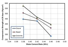
Fig.(6): Relation between Water cement ratio and Compressive Strenghth at 28 days for Different Types Aggregates
