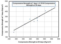
Fig.(7): Relation between Compressive Strength at 7 days and 28 days for slef Compacting Concrete
