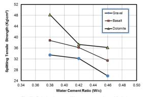
Fig.(8): Relation between Water cement ratio and Splitting Tensile Strenghth for Different Types Aggregates
