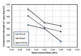
Fig.(5): Relation between Water cement ratio and Compressive Strenghth at 7days for Different Types Aggregates
