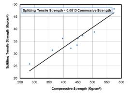
Fig.(9): Relation between Compressive Strength and Splitting Tensile Strength for Slef Compacting Concrete
