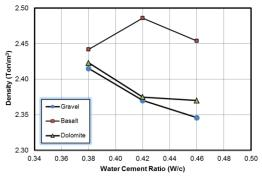
Fig.(4): Relation between Water cement ratio and Density of Concrete for Different Types Aggregates
