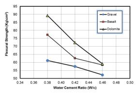
Fig.(10): Relation between Water cement ratio and Flexural Strenghth for Different Types Aggregates
