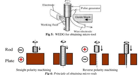
**Polarity**- The workpiece is usually set as the anode (+) and the wire electrode as the cathode(-) (straight polarity machining). This is because the discharge energy distributed to the anode is normally greater than that to the cathode.
