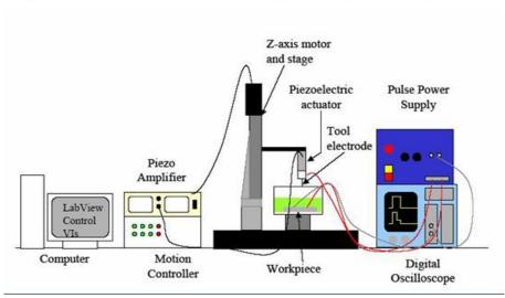
Fig 1: Ultrasonic unassisted micro EDM
