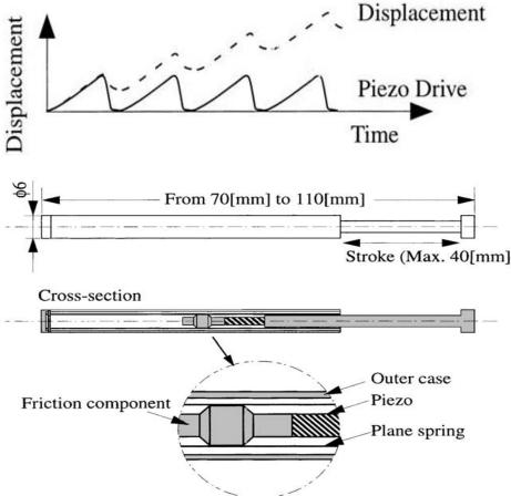
Fig 9: Micro- EDM tool feed Movement
