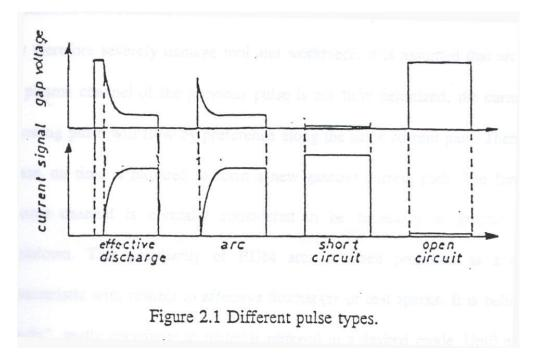
Open voltages, occurring when the distance between both electrodes is too large, obviously do not contribute to any material removal or electrode wear.
