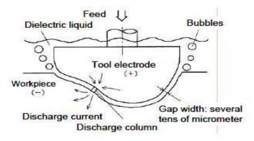
Fig 5: Micro EDM principle
