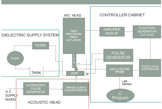
Analysis of the gap Pulses used in the EDM Process
