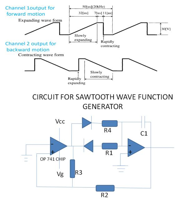
The function generator we will be using will be function generator (Wave-Factory 1946 NF). The function generator had two channel output ports. One channel (CH1) will be used for expanding the IDM actuator and the other (CH2) will be used for contracting.
