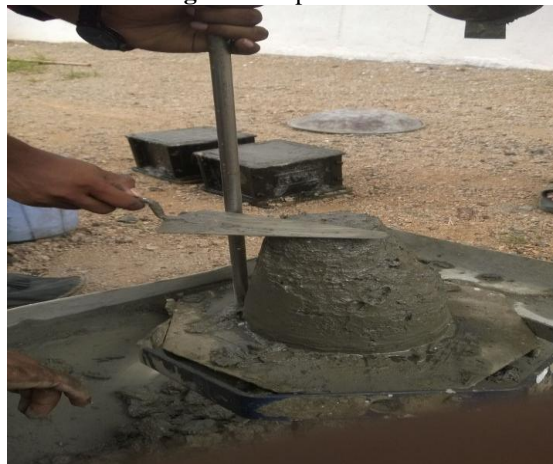
Fig 3: Slump cone test
