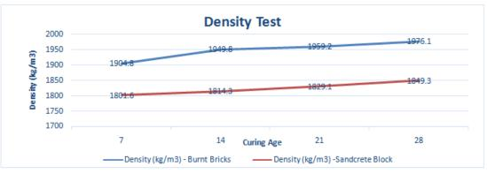
Figure 4: Density Results of Sandcrete Blocks and Burnt Bricks
