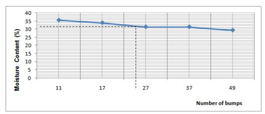
Figure 2: Liquid Limit Curve of Clay Soil
