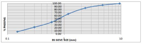
Figure 1: Sieve Analysis Curve for Sand Sample
