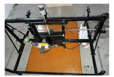
Figure 4 Actual Prototype of CNC machine
