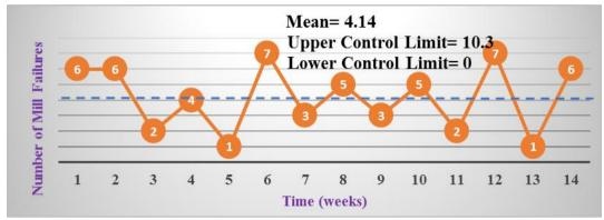
Figure 4: Statistical Process Analysis of Mill Failures
