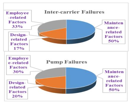
Figure 8: Assessment of Inter-carrier and Pump Failures
