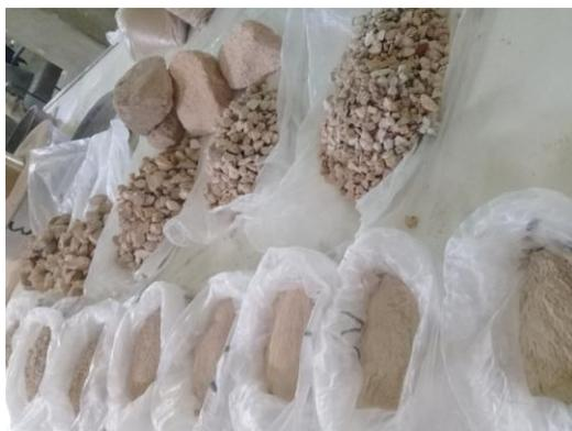
Fig (1) Recycled refractory brick after crushing and grading
