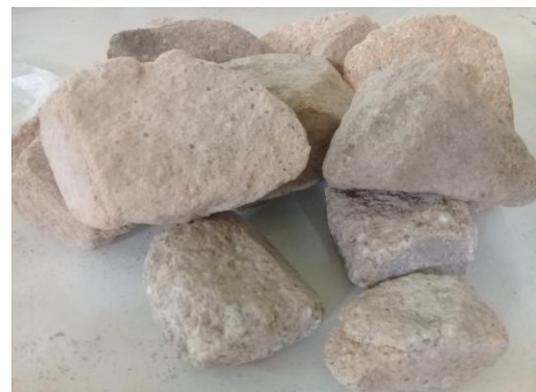
Fig (2) Recycled refractory brick
