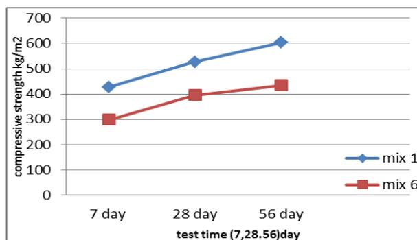
Fig (8) age of concrete with compressive strength for mix 6 (20% K, 80%F.A)
