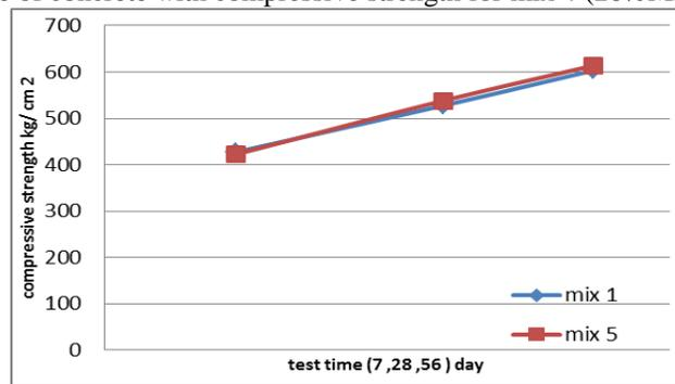
Fig (7) age of concrete with compressive strength for mix 5(20%R /80% A)
