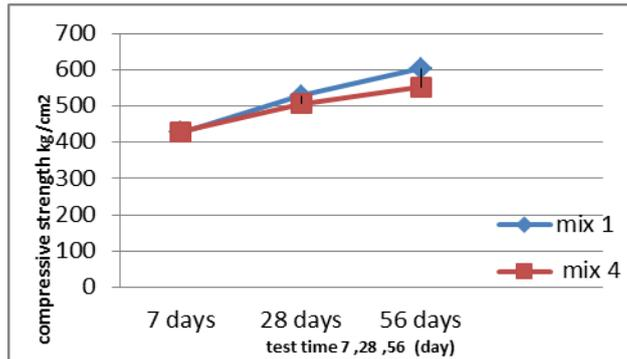
Fig (6) age of concrete with compressive strength for mix 4 (20%MK,80% F.A)
