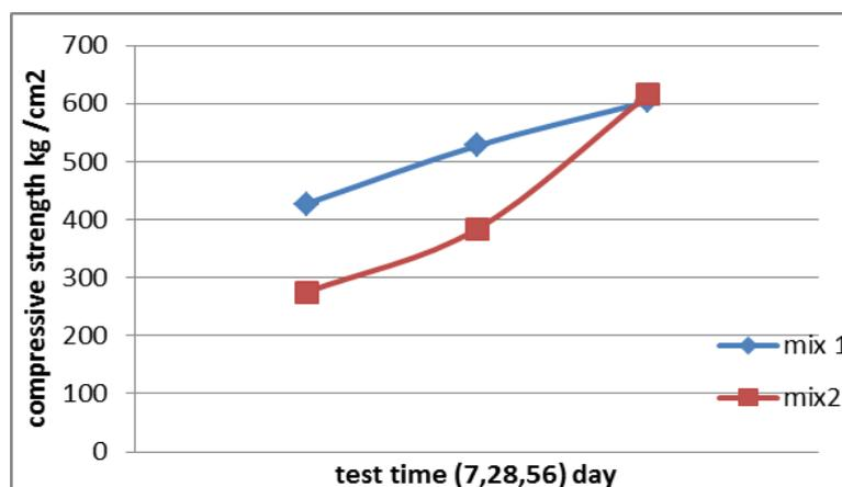
Fig (4) age of concrete with compressive strength for mix 2 (20% MK/ 80% C)
