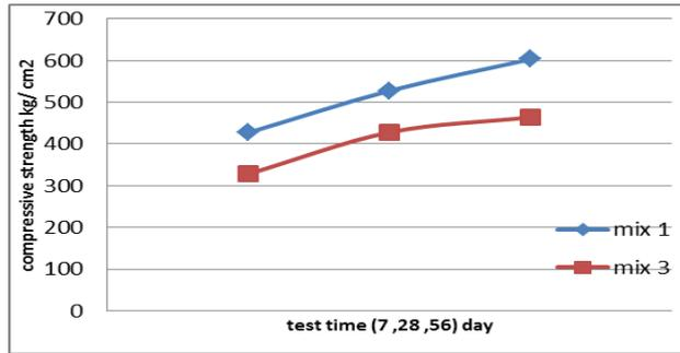
Fig (5) age of concrete with compressive strength for mix 3 (20%K,80%C)
