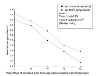
Fig 4. Superimposed Variation of flexural strength based on I.S.CodevsSFA
