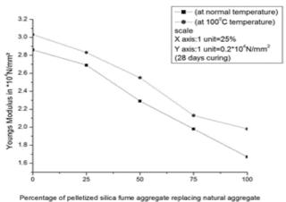
Fig 5. Superimposed Variation of young's modulus based on I.S. codevsSFA
