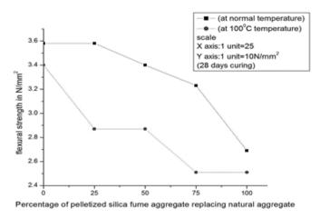
Fig 3. Superimposed Variation of flexural strength vsSFA
