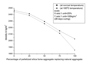
Fig 1. Superimposed variation of Density vsSFA
