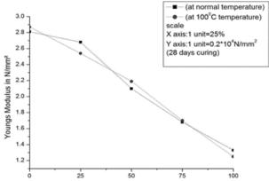
Percentage of pelletized silica fume aggregate replacing natural aggregate
