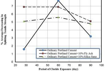
Figure 11: Relation between Period of Cloride Exposure and Percentage of Average Decreasing in Splitting Tensile Strength
