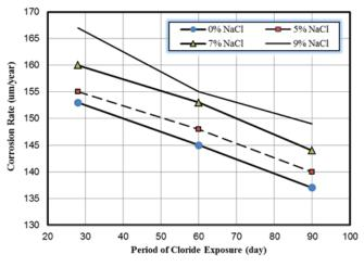
Figure 15: Relation between Period of Cloride Exposure and Corrosion Rate for Odinary Portland Cement and 10% Silica Fume
