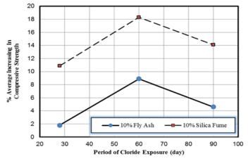
Figure 7: Relation between Period of Cloride Exposure and Percentage of Average Increasing in Compressive Strength Than Ordinary Portland Cement
