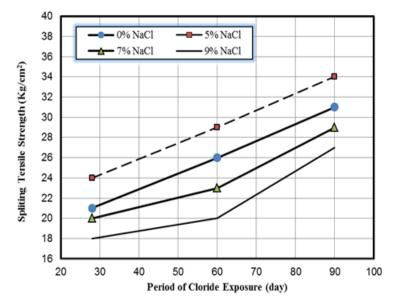
Figure 8: Relation between Period of Cloride Exposure and Spliting Tensile Strength for Ordinary Portland Cement
