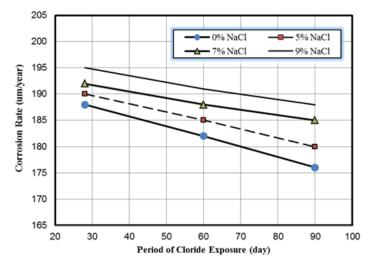
Figure 13: Relation between Period of Cloride Exposure and Corrosion Rate for Ordinary Portland Cement
