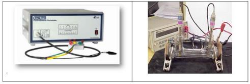
Figure 2: The Half-Cell Potential Test
