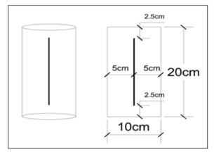
Figure 1: The Corrosion Specimen
