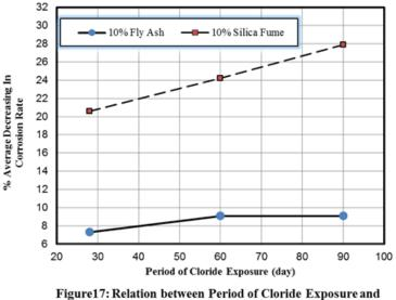
Figure17: Relation between Period of Cloride Exposure and Percentage of Average Decreasing in Corrosion Rate Than Ordinary Portland Cement
