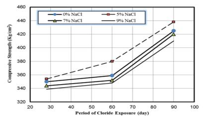
Figure 3: Relation between Period of Cloride Exposure and Compressive Strength for Ordinary Portland Cement
