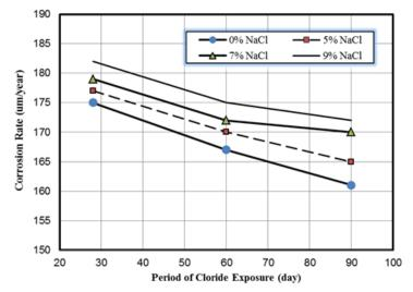
Figure 14: Relation between Period of Cloride Exposure and Corrosion Rate for Odinary Portland Cement and 10% Fly Ash
