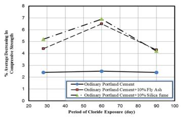
Figure 6: Relation between Period of Cloride Exposure and Percentage of Average Decreasing in Compressive Strength
