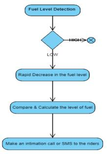
Fig.3 flowchart for detection of fuel theft or leakage
