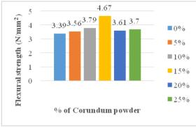
Figure 10. Flexural strength for 12 days
