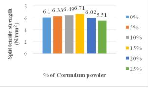
Figure 8. Split Tensile Strength For 12 Days
