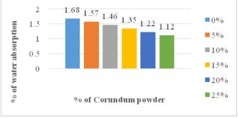
Figure 11. Water absorption percentages at 12 days
