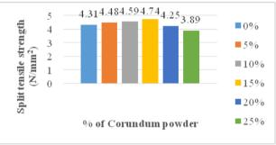
Figure 7. Split Tensile Strength For 3 Days
