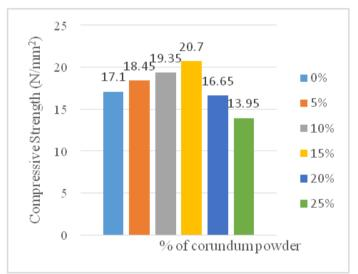
Figure 2. Compressive Strength Result For 1 Day
