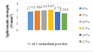
Figure 6. Split Tensile Strength For 1 Day
