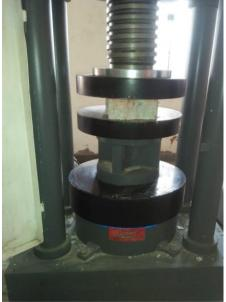
Figure 5. Split Tensile Strength Setup
