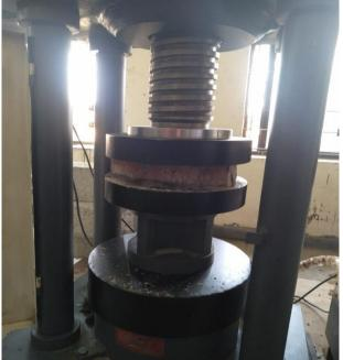
Figure 1. Compression strength test setup
