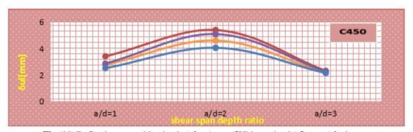
$\label{eq:fig_continuous} \textbf{Fig~(11).} Deflection~at~cracking~loads~(~dna~(mm.rc\delta Ultimate~loads)~\delta u.exp~(.for~beams~B1-1-@,~B2-1-STR,~B3-1-REP,~B4-1-STR&REP~,group~1.)~. L=92.5 CM.~B5-2@-,~B6-2-STR,~B7-2-REP.,~B8-2-STR&REP~group~2-)~. L=117.5 CM.~B9~. @3-B10-3-STR& ,.B11~3-REP&B12-3-STR&REP~.group~3-()~. L=142.5 CM~.$
