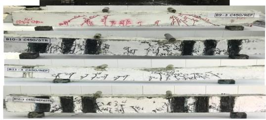
Fig: (8) Pattern of crack of beams
