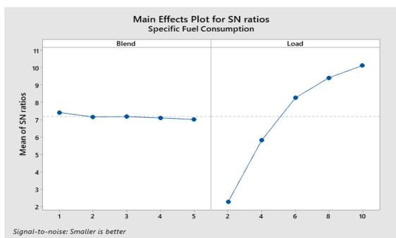
Figure 7: Main Effects Plot For S/N Ratio of Specific Fuel Consumption
