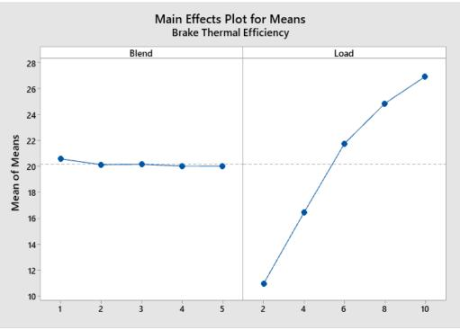
Figure 4: Main Effects Plot for Means of Brake Thermal Efficiency
