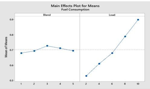
Figure 8: Main Effects Plot for Means of Fuel Consumption
