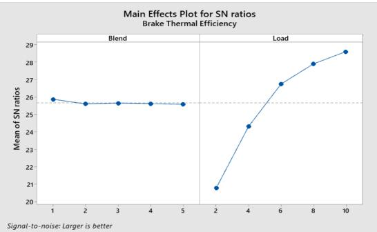
Figure 5: Main Effects Plot For S/N Ratio of Brake Thermal Efficiency
