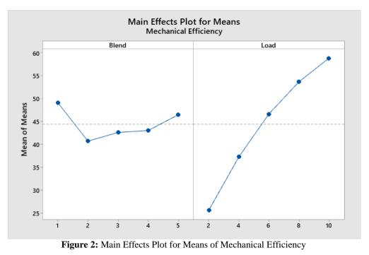
The term ideal setting is reflecting just ideal mix of the parameters characterized by this trial. The ideal setting is dictated by picking the level with the most noteworthy S/N proportion.Referring (figure) the response curve for S/N ratio, the highest S/N ratio was observed at Diesel Fuel, engine load 12 kg which are idealparameters setting for highest Mechanical Efficiency. Delta value for Mechanical Efficiency for load (7.27) and blend (1.76) shown in Table 6.
