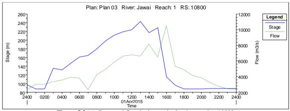
Figure 5.3 (a): Stage and flow hydrographs for river station 10800
