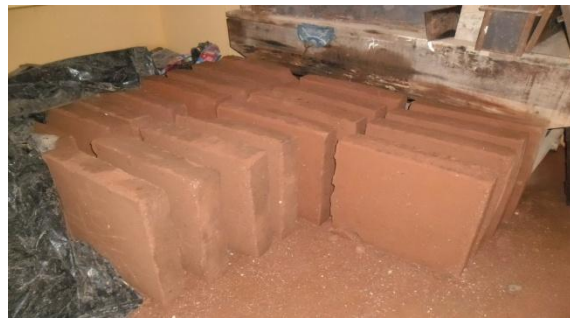
Figure 4: Reinforced compressed stabilized laterite slab
