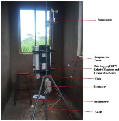
Plate 4: Experimental Set Up
