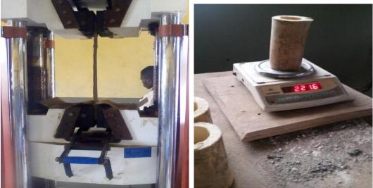
Plate 3: Tensile strength of splint bambooPlate4: Weighing Bamboo for Compression
