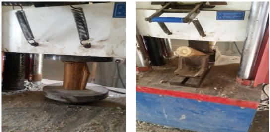
Plate 5: Crushing the Bamboo on UTMPlate 6: Flexure Strength Test of Bamboo
