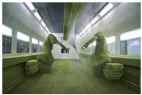
Figure 5b: trajectory painting robots
