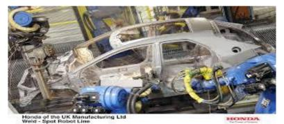
Figure12: Honda Weld - Spot Robot Line
