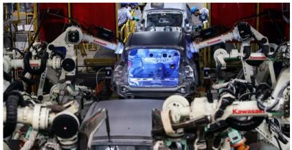
Figure: Welding robots work on cars at a Ford factory
