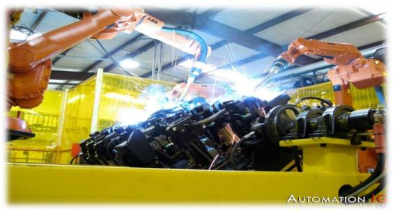
Figure8: Crown engineering robots welding cells
