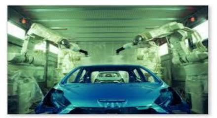
Figure1: Robotics application in automotive painting
