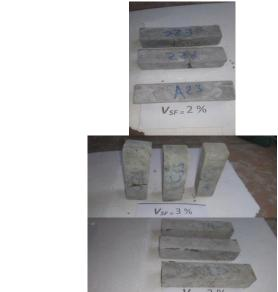
Figure 40: Impact of steel fibers percentage on shape of specimen failure in flexural strength test
