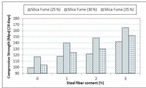
Figure 26: Impact of steel fibers on RPC compressive strength containing various ratio of silica fume at 7 days
