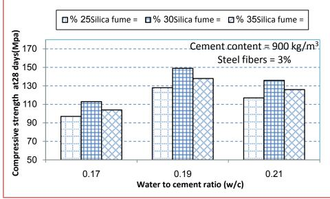
Figure 31 Effect of water to cement ratios (w/c) on Compressive Strength.
