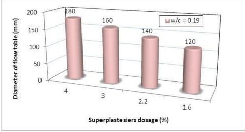
Figure 18: Relationship between of flow table and superplasticizers
