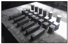
Figure 14: Concrete specimens after casting
