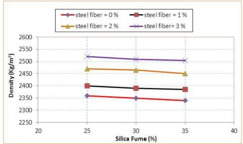
Figure 20: Impact of SF percentage on RPC density with various contents of steel fiber
