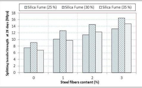
Figure 34: Impact of steel fibers on RPC tensile with various percentage of SF
