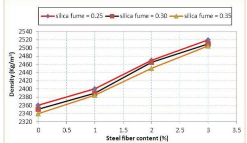
Figure 22: Impact of steel fibers content on RPC density with different contents of silica fume
