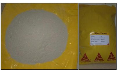
Figure 2: Silica Fume used in mixtures
