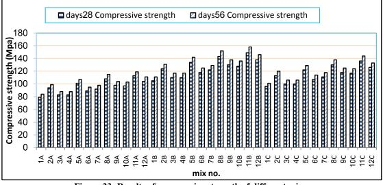
Figure 23: Results of compressive strength of different mixes
