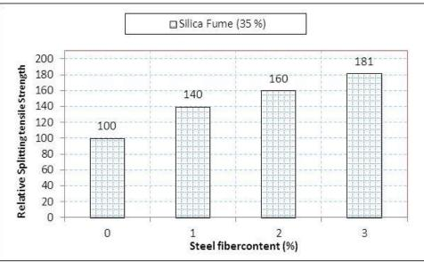
Figure 35: Relative tensile to StF with silica fume (35%)
