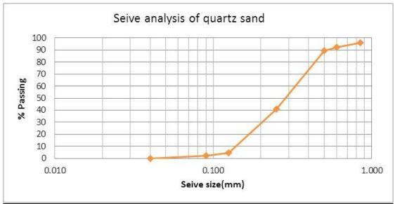
Figure Figure4: Grading of quartz sand.
