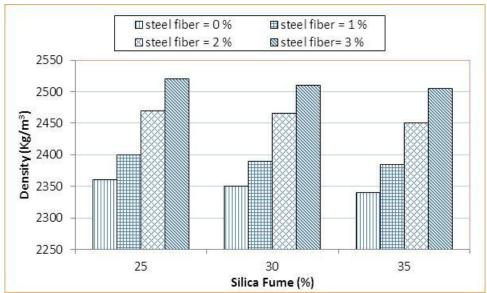
Figure 25: Impact of SF content on RPC density with different contents of steel fiber
