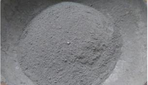
Figure 10: RPC mix after dry mixing
