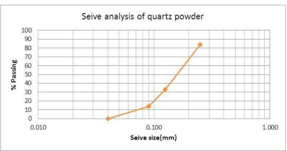
Figure 6: Grading of quartz powder.
