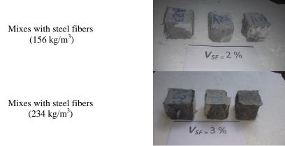
Figure 28: Effect of steel fibers content on shape of specimen's failure in compressive strength test
