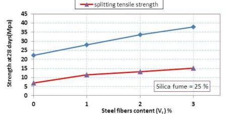
Figure 41: Relationship between tensile and flexuralstrength
