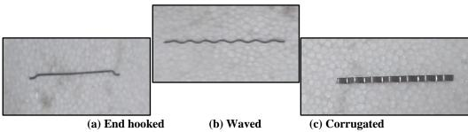
(a) End hooked (b) Waved (c) Corrugated Figure 7: Types of steel fibers available in Egypt markets
