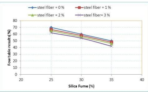
Figure 19: Influence of SF and steel fibers on flow table test results
