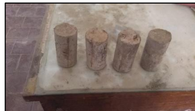
Figure 9: Effect of high temperatures (a) Partially spalled, (b) Fully failure and broke into large parts.
