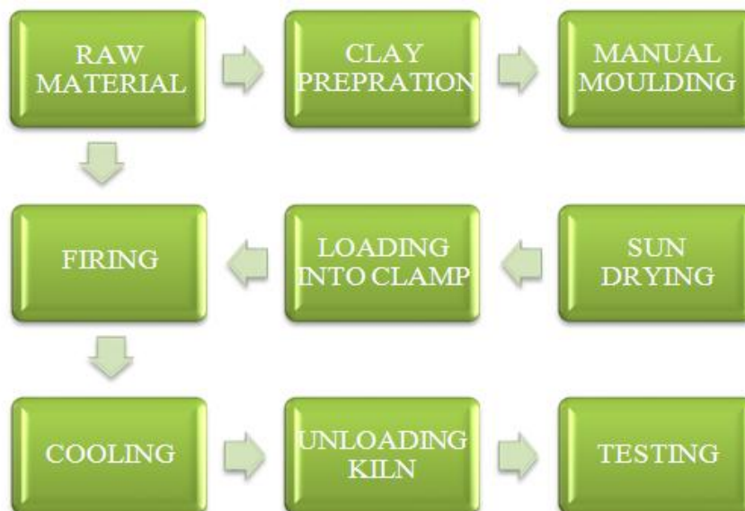
Fig. 3.7 Manufacturing process of conventional brick.
