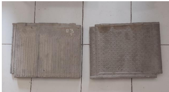
Figure 1: Flat concrete roof tile using common sand material (left) and Lumajang iron sand (right).
