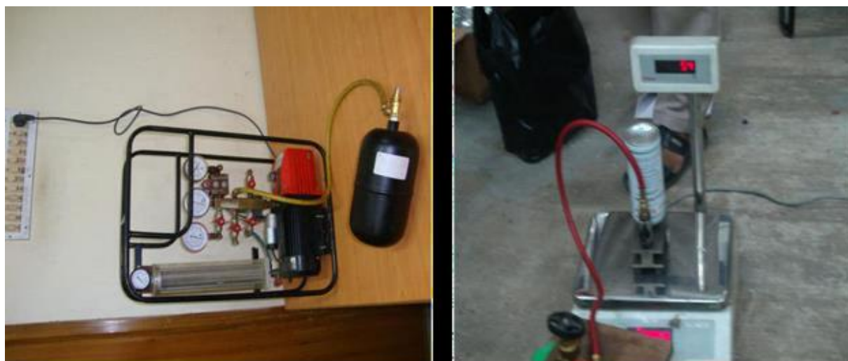
Fig 2.2 shows the charging setup of refrigerants by mass proportion
