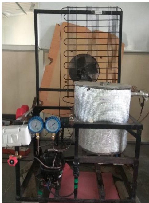
Fig 2.3 Water Chiller for Experimentation
