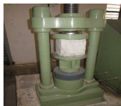
Compressive strength tests
