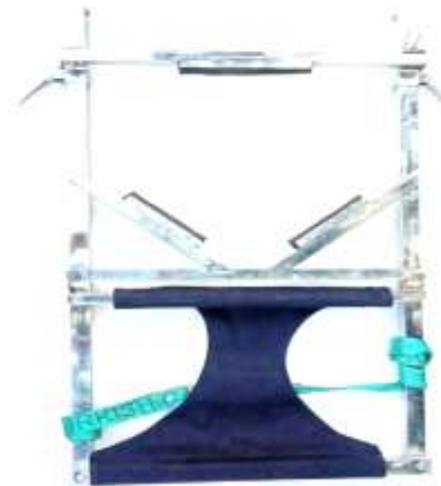
Fig. 2 Upper frame of the improved climber
