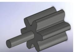
Fig 16: CAD Model of Spur Gear Pinion
