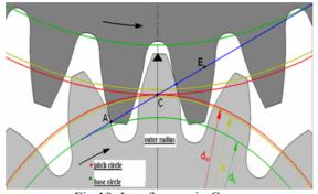
Fig 10: Interference in Gears
