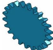
Fig 15: CAD Model of Spur Gears
