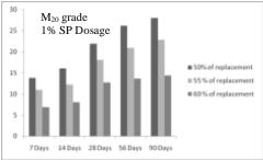
Fig.2 Effect of age and % replacement of cement on Compressive strength for 1% SP Dosage
