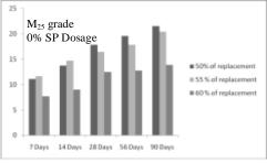
Fig.5 Effect of age and % replacement of cement on Compressive strength for 0% SP Dosage
