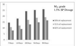
Fig.7 Effect of age and % replacement of cement on Compressive strength for 1.5% SP Dosage
