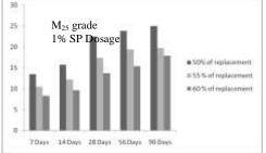
Fig.6 Effect of age and % replacement of cement on Compressive strength for 1% SP Dosage
