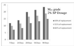
Fig.8 Effect of age and % replacement of cement on Compressive strength for 2% SP Dosage
