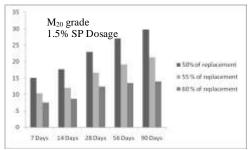
Fig.3 Effect of age and % replacement of cement on Compressive strength for 1.5% SP Dosage
