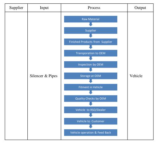
**Fig. 3:** Flow Chart – **SIPOC** Diagram
