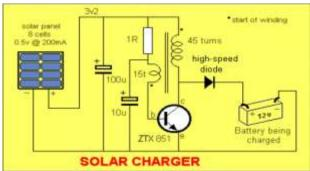
Figure 2 Circuit diagram for solar charger.
