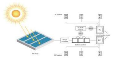
the functioning of the system and the grid and switches off the system in case of faults. **working of solar panel**
