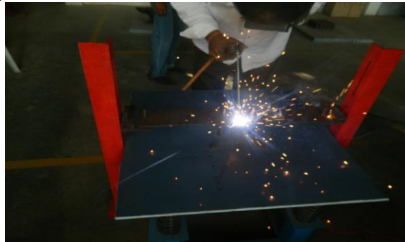
Fig.2. Welding the specimen using vibrations
