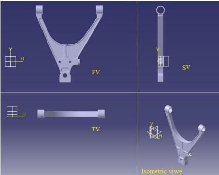
Fig. 1.1 CATIA Modeling of Lower Wishbone Arm.
