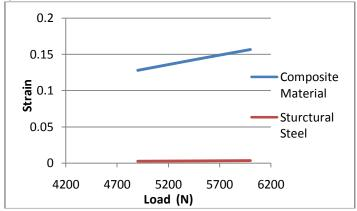
The load applied on Lower Wishbone Arm is W1 = 4900N. Then maximum & minimum total deformation values are found by ANASYS the results are given by following fig.
