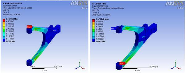
Fig. 1.2 Stress in Lower Wishbone Arm in structural steel & composite material.
