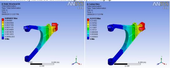
Fig. 1.4 Total deformation in Lower Wishbone Arm in structural steel & composite material.
