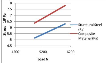
The load applied on Lower Wishbone Arm is W1 = 4900N. Then maximum & minimum strain values are found by ANASYS the results are given by following fig.
