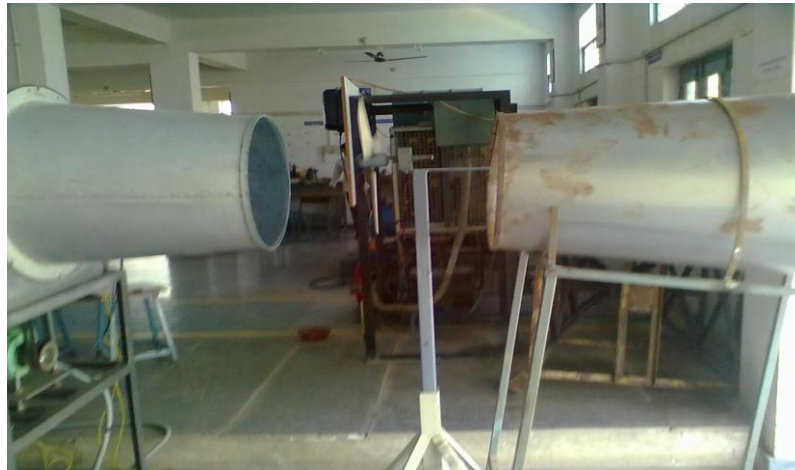
Figure4: Wind Turbine And Using Diffuser Augmentation In Combination With A Convergent Nozzle
