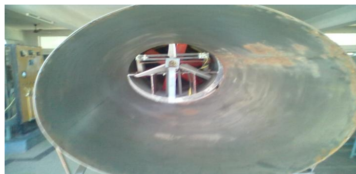
Figure7. Abut View Of Rear End Of Diffuser Augmentation And Combination With Convergence
