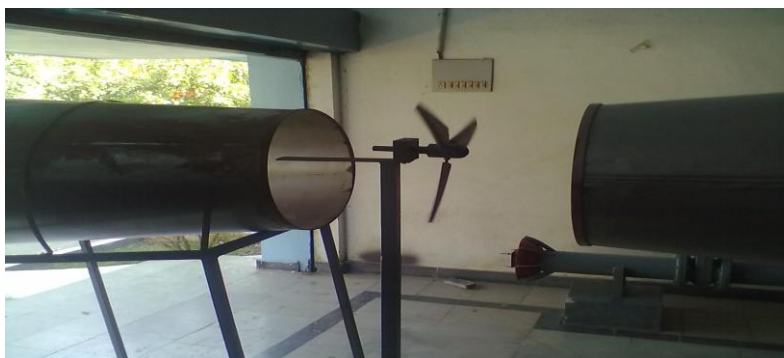
Figure6: Right Side View Of Diffuser Augmentation And Combination With Convergence
