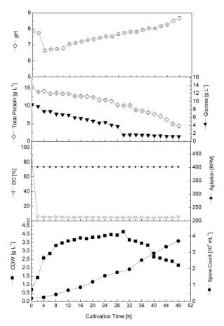
Figure 2. Cell growth, glucose consumption, spore production and change in pH during Bti cultivation in batch bioreactor under uncontrolled pH.
