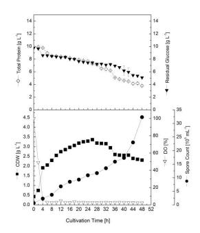
Figure 3. Cell growth, glucose consumption, spore production and change in pH during Bti cultivation in batch bioreactor at Controlled pH.
