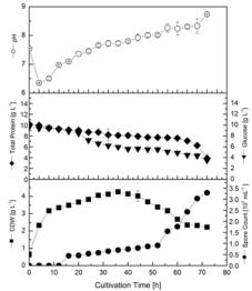
Figure 1. Cell growth, glucose consumption, spore production and change in pH during Bti cultivation in shake flask culture
