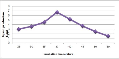
Figure 5. Effect of different incubation temperature on the lipase production by the selected isolate HM10
