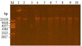
Lane 1-10: Plasmid profile of *E.coli* isolates isolated from clinical samples Lane M : Lambda DNA Hind III digest - DNA marker
