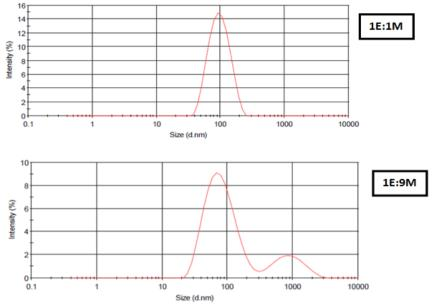
Fig 4: DLS bar graph of silver nanoparticles synthesized with different concentrations
