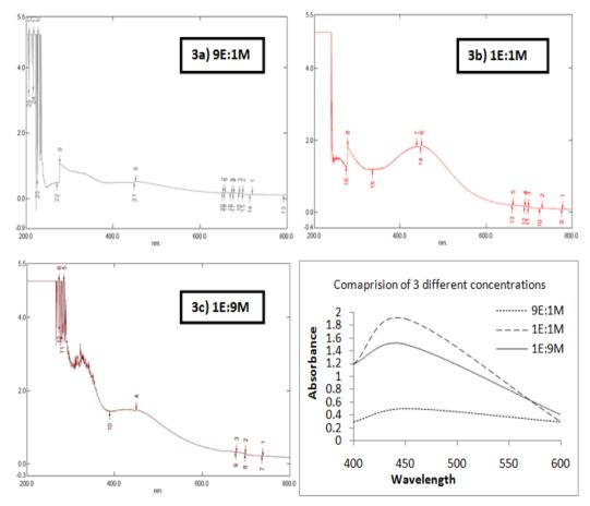
Fig 3: UV-visible spectra recorded for reaction mixture of three different ratios of plant extract (E) to metal salt (M)
