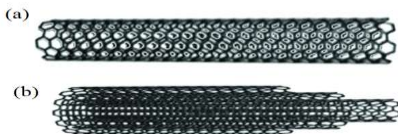
Fig. 8 : : Molecular representations of (a) SWCNTs and (b) MWCNTs
