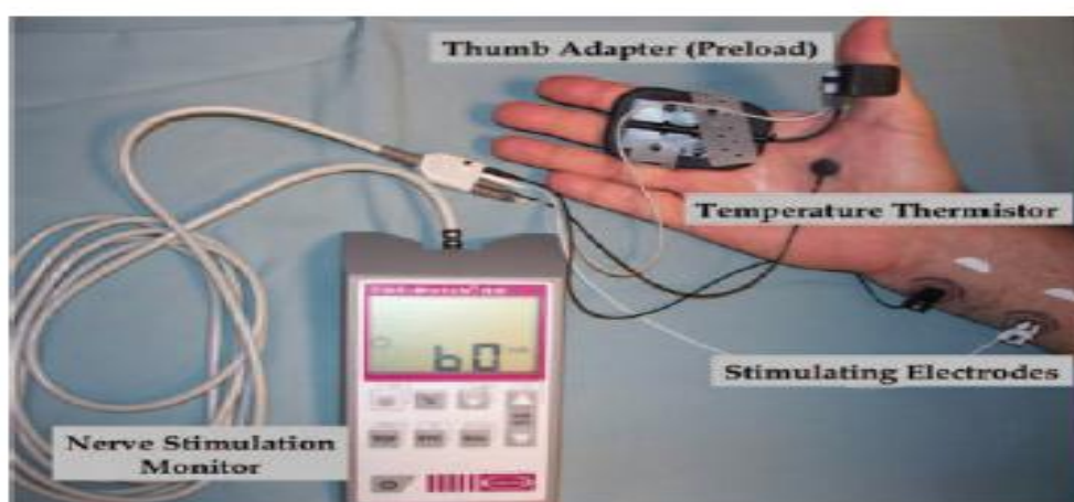
Figure 4. Example of acceleromyograph (AMG). The thumb movement in response to ulnar nerve stimulation is sensed by the piezoelectric sensor that is fixed to the thumb via the thumb adapter, and the acceleration (which is proportional to the force of muscle contraction) is sensed by the interfaced monitor. The current amplitude is displayed by the AMG monitor (60 mA on the screen). To improve the consistency of responses, the piezoelectric sensor is fixed to the thumb, which is placed under slight tension (200-300 g, "preload") by the thumb adapter.
