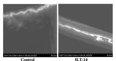
Fig. 6. Appearance of the SEM results of polypropylene, polypropylene control plastic before biodegradation test and ILR-14 polypropylene plastic after degradation at 20.00x magnification.
