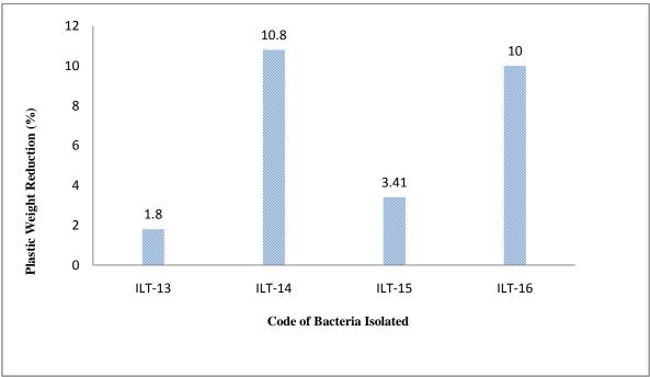
Fig. 1. Biodegradation Test of Polypropylene Plastics by isolated bacteria from Seawater
