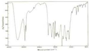
Figure 2. IR spectrum of aristolochic acid
