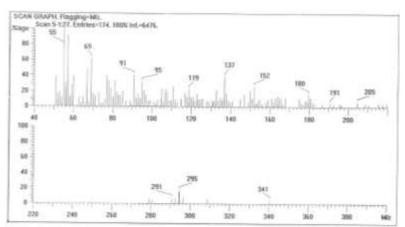
Figure 6. Mass spectrum of aristolochic acid
