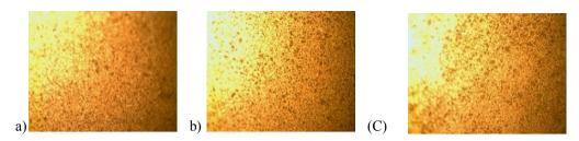
Fig. 6 Microstructures of medium carbon steel austenitized at 900<sup>o</sup>C, quenched and tempered at 350<sup>o</sup>C a) (mineral oil; b) neem oil; c) watermelon oil x200.
