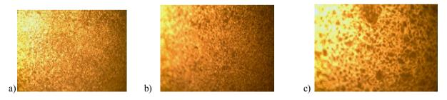
Figure 5 Microstructures of samples that were austenitized at  $900^{\circ}$ C, tempered at  $300^{\circ}$ C with the tree quenching media. a) mineral oil; b) neem oil; c) watermelon oil x200.
