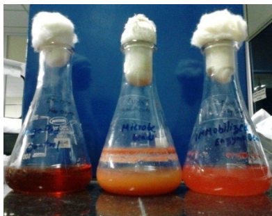
Fig.15.Dye decolorizing activity of immobilized Penicillium chrysogenum and enzyme with control (0.01%) congo red dye solution
